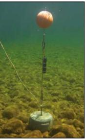
AN ACOUSTIC receiver anchored underwater. More than 3,000 receivers in the Great the process of detecting signals from fish implanted with individually coded acoustic transmitters. (Photo credit: T. Binder, Great Lakes Fishery Commission via GLATOS)
